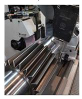
• Single diameter in-process measuring systems
